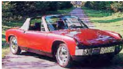
The mid-mounted engine layout offers an almost ideal weight distribution. This two-seater with the pop up headlights and the removable plastic roof was in special demand on the US market.
